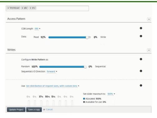
A profile that emulates the workload of the application and then iterates the test over various queue depths could be generated. Block sizes were also altered since block size may have an impact on bandwidth and IOPs (variables in the grey columns below).
