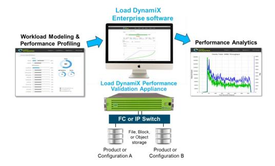
The Load DynamiX platform provides comprehensive storage workload modeling and performance validation, enabling storage architects, IT operations personnel and storage engineers to optimize the performance, availability and cost of the storage infrastructure. The platform supports all file, block and object storage protocols and is comprised of two components: the Load DynamiX Enterprise software and the Load DynamiX Performance Validation Appliances for extreme storage load testing.
